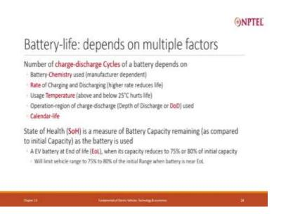
When capital costs are high, how long will the battery last? The life cycle of the battery becomes extremely critical. If the life cycles are small, we have to put that large capital cost again and again, if the life cycles are larger, I do not have to invest that on the battery again and again. So, the key parameter one of the most important parameters is, what is the number of charge-discharge cycle that a vehicle can support?
