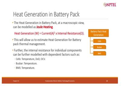
Then we have also talked how heat is generated in a battery pack, so the simplest form of the heat generation which can be written in mathematical form is Joule, like Joule heating is nothing but I square R, so I square is the current drawn from the battery or current fed into the battery during the charging, current drawn from the battery during the discharge and the internal resistance of the cell.
