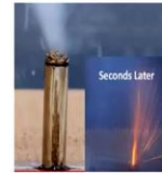
Cell Thermal Runaway, a Safety Concern. Initially, Venting of Gases occur, followed by High Temperature Explosions.
