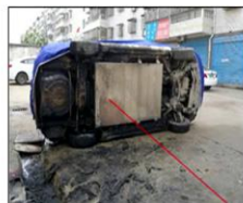
Battery Pack Intact after Crash. Source: SteelGuru.com
