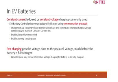
So, constant current followed by constant voltage charging commonly used EV, now electrical vehicles will constantly communicate with charger. So, the vehicle has a battery, there is a charger the two will be talking to each other. And saying no-no-no my current is becoming like
