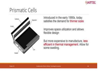
Prismatic cell; this was introduced in 1990s. And prismatic this is the one which is very thin. How thin? Much thinner than a cellphone about a third, no way half, almost half as much. So and since it is stacked on top of each other, it improves the cell utilization,
