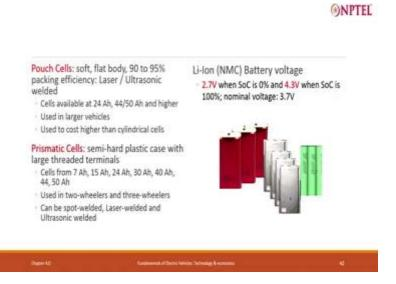
So, this is what the pictures are, this is the cylindrical cell, this is a pouch cell and this is prismatic cells. The pouch cell is soft, flat body soft. You will in fact, twist it if you want ofcourse it will destroy the battery. It has a very high packing efficiency.
