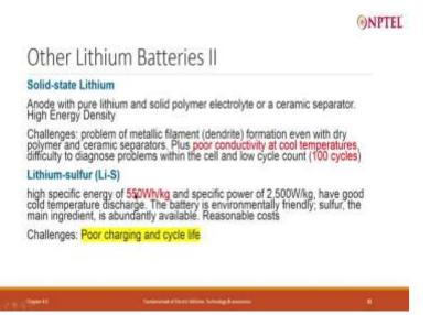
Lithium sulphur better in terms of energy density poor charging and cycle life.
