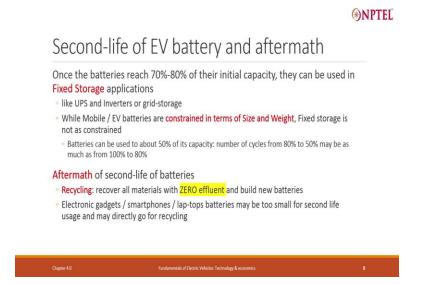
There is a second life of the battery that after the battery capacity has gone down and you no longer want to use in electric vehicle you can still use it somewhere else for example in fixed application where you do not mind the battery size to be little larger, so you actually keep it and for example UPS and all that and of course I had mentioned that aftermath of second life is you want to recycle, we will come to that later on.
