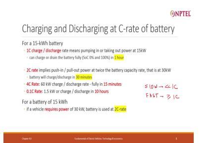
There is a very important concept that I have been talking about repeatedly the C rate of the battery. It is defined as how many C, 1 C, 2 C, 0.5 C, 1 C charging or discharging rate basically means the battery could be charge from 0 percent to 100 percent SOC in 1 hour. So, that is the 1 C, 2 C basically means half the time twice that rate, so actually you can charge from 0 percent to 100 percent in 30 minutes and 0.1 C will mean it will take you 10 hours to charge from 0 percent to 100 percent.
