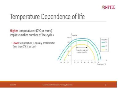
Then I sort of said that higher temperature impacts the life of the battery, lower temperature effects the life of the battery, a minus temperature does impact the life of the battery, you like it to operate probably between 15 degrees and 35 degree centigrade, again it will depend on battery to battery, you will buy from manufacturer 1, who may say this is the optimal place another one will say another optimal place is something else.
