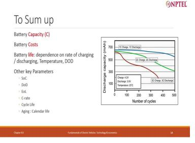
So, to sum up, we had talked about battery capacity and battery costs are the two important parameters, it will depend on the battery life because finally usage cost depends on the battery
