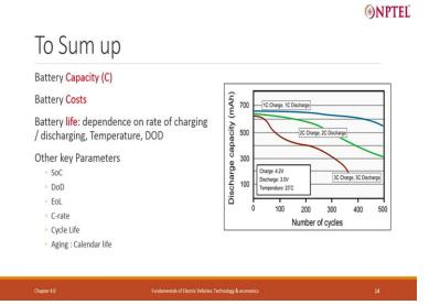
To sum up, what have we done so far, we have defined battery capacity, we have always said battery costs are very important we will look into it that more detail, battery life dependence on rate of charging discharging, temperature and depth of discharge, look at this, this is 1 C charge 1 C discharge and you see discharge capacity 1 C charge discharge, in 500 cycles the battery life goes down, but it looks like the battery will last for at least another 5 minutes cycles 1000 cycles.
