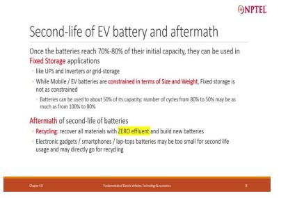
Second life for the battery, once the battery reaches 70 to 80 percent of the initial capacity it can be used for fixed storage, weight is not a constraint, volume is not a constraint, like UPS or inverter or grid storage. Electric vehicle is always constrained in terms of size and weight and whereas fixed storage is not.
