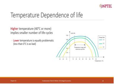
Higher temperature or lower temperature as I said effects the battery life, battery life is ideally between 20 and I will say 15 and 35, 15 and 35 it is okay, it deteriorates not as bad, but if you see even the deterioration is more at 3 C rather than 2 C and 1 C, 1 C it may handle larger temperature range and 2 C does not handle as much, 3 C it handles much less number of life cycles can go down like anything.
