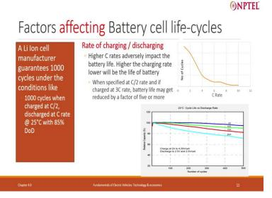
Factors affecting battery cell life, a lithium-ion battery manufacturer may tell you that I am giving you a battery cell which lasts for 1000 cycles, but they will always define, that the 1000 cycles is charging at C by 2 rate, discharged at maximum 1 C rate and always at 25 degree centigrade with 85 percent depth of discharge.
