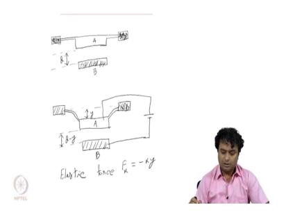
So, in the last class, we were discussing about the system which is a coupled system. Coupled system means that it is also attracted by the electric field as well as the mechanical force or the electrostatic force is trying to pull the A plate up. And in that case, we have already seen that.
