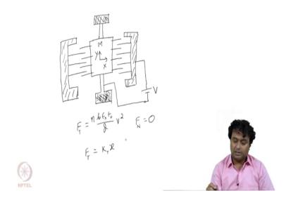
So, what is a comb actuator? comb actuator is a structure like this. So, we will draw the structure. So, this plate is fixed at this to support. So, this shaded region at the points or at the
