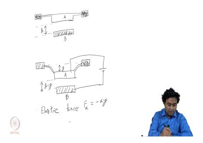
Now, once we know some basics of electrostatics we will try to couple the electrostatic force with the mechanical force, what we learnt in our previous modules? So, I am first drawing two different cases. So, this is a fixed plate let us say this call this A and B. So, A is A is a plate which can move ok. And, this is supported by 2 beams which are connected in the opposite direction by some fixed support as it is shown by this shaded area. And, this B plate is already fixed at the bottom ok.
