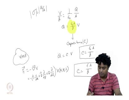
Now, this epsilon naught A by d, this term is known as capacitance C, capacitance C and if we put this c then we will get that Q equals to C into V, where C is equal to epsilon naught A by d. So, this is the expression for the parallel plate capacitor and then if we have a say here, in between in between the parallel plates, if we have any dielectric material of let us say some dielectric constant epsilon, then this expression will come as C equals to epsilon A by d ok.
