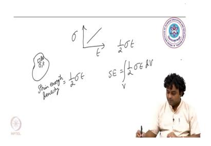
So, now, you know that according to laws of elasticity stress and strain are linear right. So, if the sigma is the stress and let us say epsilon in the strain, then you get a linear curve. Now what is the area under this curve is half into sigma into epsilon and this is also known as the strain energy. This is also known as strain energy.
