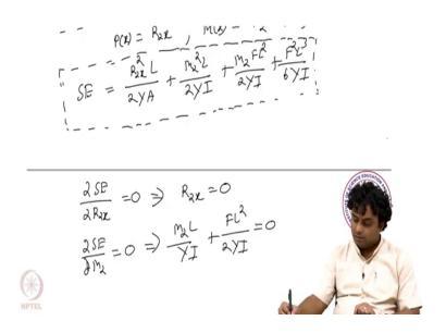
So, delta SE by delta R 2 x equals to 0 lies that R 2 x equal to 0 because in this strain energy team, this energy term the only term which depends on R 2 x is R 2. If the first time R 2 x square L into L divided by 2, I A the other terms are independent of R 2 x. So, that will become directly 0 ok.
