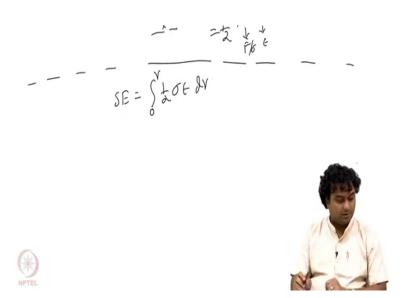
So, total strain energy SE is equal to integral 0 to volume half into sigma epsilon dV ok. Now we will discuss a theorem called Castigliano's theorem.
