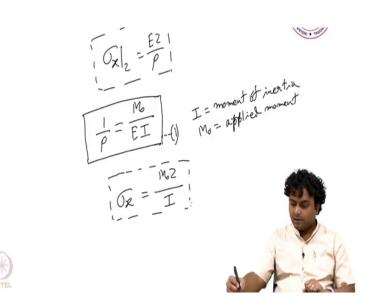
Now we are going to use this relation for our current solution. So, M 0 z by Y where M 0 is was the moment and z was the deflection from the neutral axis. And here in this case, we are considering this as w right because in Y direction or in the vertical direction, we are considering the deflection as w.
