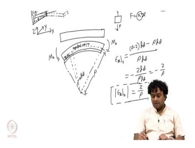
Here you can see that this is the case where it is pure bending. So, there is no lateral deflection associated with it right; neutral axis and according to the neutral axis is pure bending case for this transfers force cantilever right. But here what we are considering now? We have axial stress also and transfer stress also because this is guided case and then we have to calculate the strain energy for both the cases.
