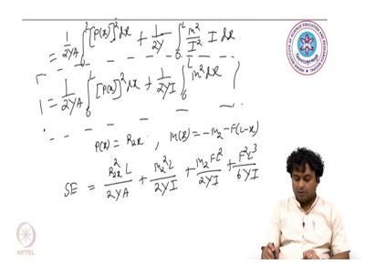
Now putting these two equation that is P x equals to R 2 x and M x equals to minus of M 2 minus F into L minus x. We put these two equations on in the strain energy expression to guess strain energy equals to R 2 x square into L by 2YA plus M 2 square L 2YA 2YI; 2YI plus M 2 2F of L square divided by 2YI plus F square L cube divided by 6YI. So, this you can get by just putting the M values and the r R 2 x and integrating it.
