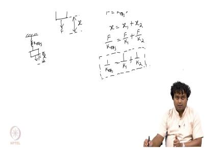
Now, if the system is modeled as an equivalent system we have only one spring constant right, and then one single mass also will have a force of F. And then this, let us assume this is K equivalent s. Last one let us assume this is K equivalent p or parallel and this is s for series. So, then you can write that F is equal to it will have the same total deflection right x same total deflection x. So, F is equal to K equivalent for series into x.
