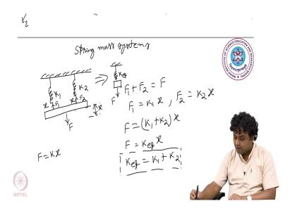
Now, we will see spring mass system. We have seen that; let say we have spring and mass connected to that, then you can simply write that if the displacement is let us say x and force acting is F, the spring constant is K then f is equal to K x. Now, and we are going to model our systems like this spring mass system. So, that we can directly use the K value and accordingly we can solve any problem.
