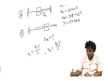
K 1, K 1 means the thinner beams and K 2 is the thicker beam let us say. K 1 is equal to A 1 Y by L and K 2 is equal to A 2 Y by L.
