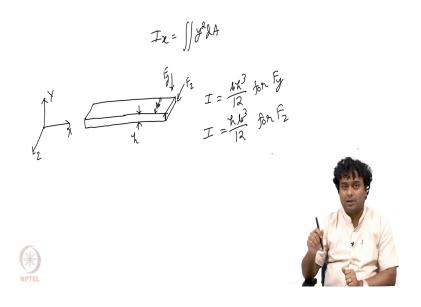
Now, let us consider the beam geometry we have. If we are considering the force; first of all for this kind of geometry, the inertia I can be written as b h cube by 12. Where b is the width or breadth and h is the height. And we are not going into the derivation of this expression, because this is not part of this course, ok so that you can find out from simple mathematics or mechanics.
