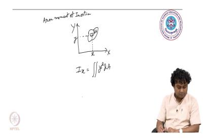
So, let us assume that this object or this area is at a distance x comma y in this rectangular coordinates system. Now, area moment of inertia is defined as like what is the moment? Moment is that how far is the area from some axis. And let say if we are calculating the moment of inertia with respect to the X axis then from X axis it is at a distance of y. So, I x is defined as area integral of y square, ok.
