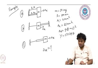
So, now we will see one example based on the concept whatever we have discussed. So, there are two beams, ok. There are two beams and these two beams the length of the beam is same, but the area of cross section is different, ok. So, let us assume this l, and l is the length and A l and A 2 is the area of cross section.
