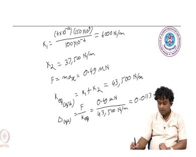
And if you put the values then you will get K 1 equals to 4 into 10 to the power minus 12 into Y is 150 giga Pascal so, that is into 150 into 10 to the power 9 right and then L 1 is 100 micron. So, that is 100 into minus 6 equals to 6000 Newton per meter. And similarly K 2 will be how much, K 2 will be just here it will be 25 and it will come as 37500 Newton per meter, ok.
