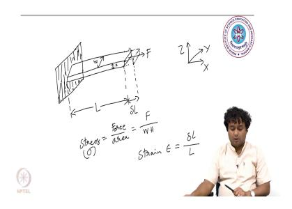
Now, we will discuss different constants. And constants means like for a beam structure and applied forces what kind of constant are applicable for that particular beam; means, what motions are allowed and what motions are not allowed. Like for this structure you can see that for the left hand side there is no motions are allowed like X direction Y direction Z direction no motion are allowed as well as rotations are also not allowed, right.
