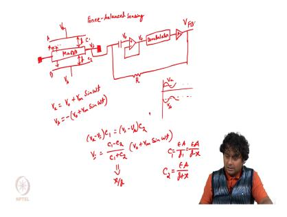
Now, let us say, we will see that, how we can use this kind of capacitive measurement for force balance sensing. This is force balanced sensing; means the force will be balanced. So, what does that mean? We will see. So, let us say that, there is this proof mass, which can move in on the vertical direction only ok. So, it can this proof mass can oscillate in this direction; in this direction.
