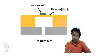
Now, what is the basic concept of this pressure sensor as we have shown that, there is a pressure port through which the which is connected to the membrane and as we apply some pressure the membrane deflects, right. Because it has in this region the pressure is different from compared to this region. So, the membrane will deflect. Now, we can put some sensing element on top or some sensing technique to measure this deflection, right and accordingly we can measure the pressure.
