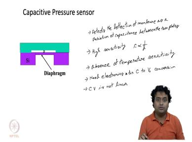
Next is capacitive pressure sensor. So, in capacity pressure sensor; we again we have the same kind of arrangement. So, we have a diaphragm like this and on the top side also we have a plate. Now, as let us say this is actually connected to the bottom side is connected to the pressure port.
