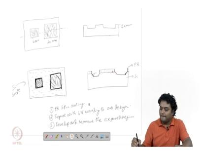
So, let us see; let us assume this is the structure we need to create. So, this is the structure I am; I will be drawing both the top view and the cross sectional view. So, while you are making this kind of diagrams or designing any of this kind of devices, we need to understand; what is top view and what is cross sectional view.
