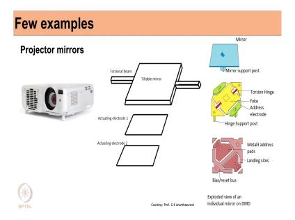
To give you some examples of MEMS devises, right. The first example is like this projector mirror. So, these are tiltable mirrors which tilting angle you can control using electrical signals or pulses and in this case, this tilting angle will decide that where the pixel will form and what will be the intensity and colour of the pixel etcetera. So, there are like thousands of this micro mirrors which are working inside a projector to make the picture projected on your screen.
