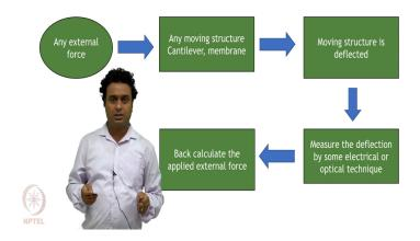
Finally, I will end this module with this slide that is general working principle for MEMS sensor. You take any MEMS sensor it can work following this general principle. So, there is some external force which is applying on some moving structure. So, let us assume this is like a cantilever which fixed is this that at this end free at this end, right.
