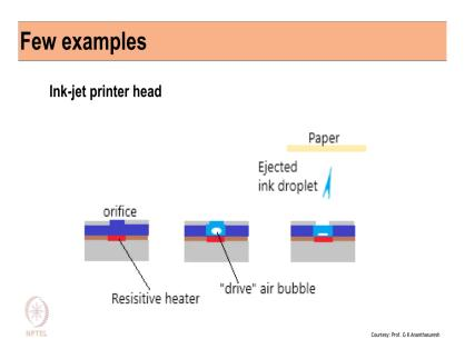
Then, an ink-jet printer; what is an ink jet printer? So, as you can see; so there is an orifice through a hole and then you have your ink which is surrounding a bubble. Then you have a resistive heater. So, as you pass some current it heats up and the bubble or the air bubble burst and that shoots out the ink on the paper. So, this is how ink jet printer head works, this is also product of micro technology or micro electro mechanical system.
