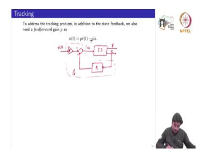
So, to address the tracking problem in addition to the state feedback, we also need a feedforward gain p defined by this. So, now, if you see a structure of the state feedback system this is the state space system where we have two outputs let us say y.
