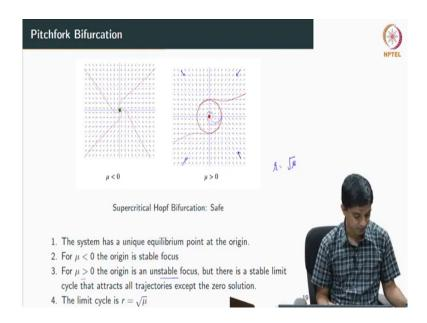
When mu less than 0 what I have is that the origin is a stable focus all trajectory spiral to the origin when mu greater than 0 this becomes an unstable equilibrium. But what happens is all the trajectories go and converge to a limit cycle whose radius is given by r equal to square root of mu, ok. For mu greater than 0 origin is unstable, but there is a stable limit cycle that attracts all trajectories except the 0 solution, right.
