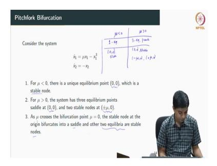
What happens is look at for mu less than 0, ok. And if I look at 0 comma 0 is stable and for mu greater than 0 I will just call it (Refer Time: 21:20) reverse is a saddle, ok. Now, similarly the point mu comma 0 when mu is less than 0 is a saddle and this is stable for mu greater than 0.
