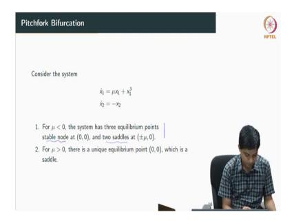
So, for mu less than 0, I will have 3 equilibrium points, a stable node at 0, 0 and two saddles at plus minus mu comma 0, ok.
