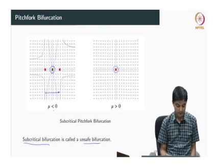
So, I have picture, right, yeah. So, for mu less than 0 this is stable. So, this is all good now these two are unstable, ok. Assume this is my operating point and a sudden change in parameter or sudden change in conditions pushes the parameter from mu less than 0 to mu greater than 0. What you see is that these two red dots which were appearing here they disappear.
