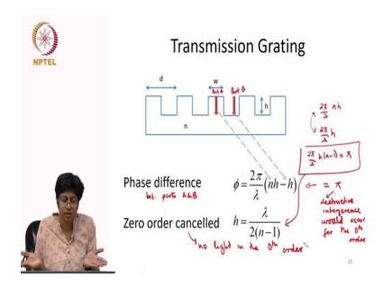
So, how do we do this to help us figure out efficiency? Let us consider a beam that is incident and we are only now looking at a part of that beam the path that travelled through this section of the gratings. So, it went through a height h of refractive index n, so the phase seen by this part of the beam is  $2\pi/\lambda * nh$ .
