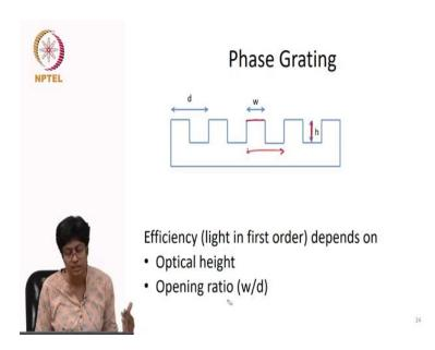
So, this construction tells us when light is incident on a grating and what is a grating a collection of periodically spaced slits they may be amplitude slits they may be phase slits. When light is incident on such a structure it breaks up the light and sends it into very specific directions called orders of the grating and those orders are determined by the period of the incident angle and the wavelength of the light.
