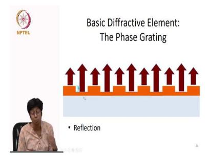
These are both examples for transmission elements I could have reflection elements, but the optical path length is now. Because this light though both sets are reflected this is reflected after going through twice this distance, so it goes down and it comes up so it has travelled twice a distance more than these beams.
