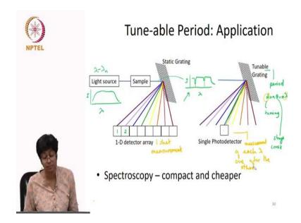
So, I could create a tunable grating. Why would I need to do that? Look at an application that let's go back to spectroscopy. I have a light source; that means I have a range of wavelengths those different wavelengths are going through a sample and from the way the wavelengths change through the sample.
