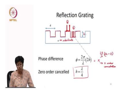
I can use a similar idea for a reflection grating here part A of the beam hits this surface and reflects here whereas part B travels this distance h and then another distance h and comes
