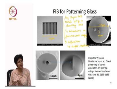
And I will end with just some pictures showing you some structures that we have fabricated here. So, this is a blazed grating. You can see this scale represents 5 microns so this is about 10 microns. So, that is the size right this is actually a grating a circular grating fabricated on a fibre tip so this is the diameter of this it is a fibre. So, the diameter is 125 microns again this is roughly 10 micron diameter and these are some other kinds of elements also fabricated on fibre.
