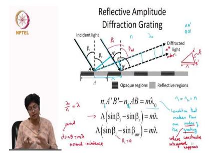
So, how do we arrive at the grating equation? I have a beam of light that is incident. And now let us just take two extremes of this beam: the one that hits this point and the one that hits a point corresponding to one period away.
