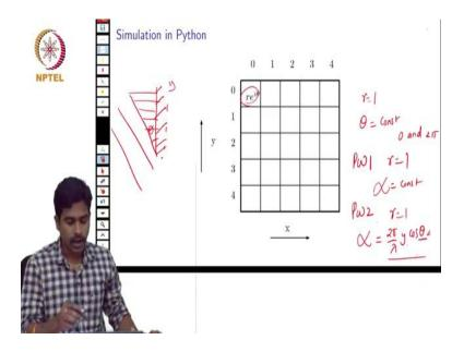
So, first of all there are 2 plane waves and we have to represent each of these plane waves as a matrix in python or an numpy array which we have seen in the previous lectures ok. So, if you look at this picture for the first plane wave the phase along this screen is constant because it is going parallel to the screen.
