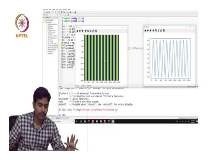
So, we got two figures so the first figure is actually an intensive interference pattern and the second one is the one of the rows I have taken from this figure and then I have plotted it to show the sinusoidal variation. So, this is for the case where the plane waves are going at 1 degree with respect to each other. So now, can you guess what happens if we increase the angle? Can somebody answer?
