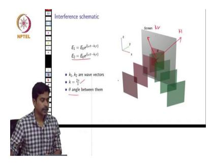
So, before that let's look at the interference between 2 plane waves, so in this figure there are 2 plane waves travelling in two different directions. So, the red one is travelling in this direction and its wave vector is given by  $k_1$  and the other plane wave shown in green color, it is travelling in some in this direction and its wave vector is given by  $k_1$ .
