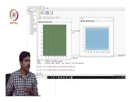
So, as you can see from this, the number of fringes have increased a lot compared to the previous case. So, one observation we can make from this simulation if the angle between the plane waves increases. So, the number of plane waves also sorry the number of fringes in interference will increase.
