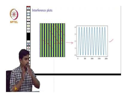
So, this is the interference pattern image, so which has a sinusoidal variation. So, what I have done in this adjacent figure is I plotted the intensity along one of at the midpoint of some, some one of the rows I have taken from this figure and then I have plotted in this graph.
