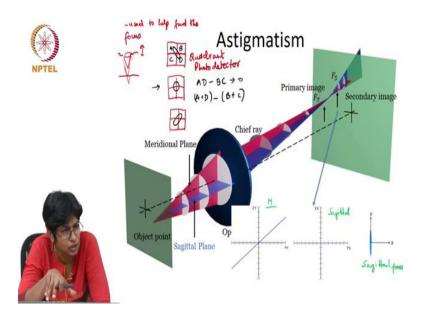
So, astigmatism can be used to help find the focus. So, the CD and we will look at that in more detail, but basically the CD system and other similar systems have a lens which has the ability to move up and down ok. So, you can control that movement. Now as its moving you are changing where the focus may be the focus happens here then you move it down then the focus will happen here if you move it further down the focus right.
