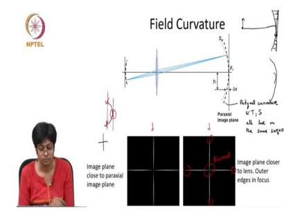
Now, the final aberration we look at is field curvature. So, again if we go to an off axis point it should not be surprising that the ideal image surface is not actually a planar surface, but a curved surface right we have always been talking about I if you have an optical system if you have an object then and I look at let us say I have an object which has some height.
