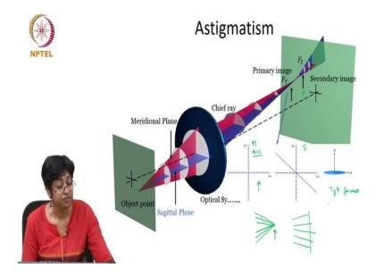
Another line, but will the lines be exactly the same? So, maybe this image helps you a little bit, in this case I am my focus; so, I am now looking at the tangential focus, this is the line which is basically caused by all the sagittal rays right. So, the tangential rays have come to a point focus, but the sagittal rays are spread out and I get a line like this. What will I see if I look at this surface? It is still a line, but it is a vertical line ok.
