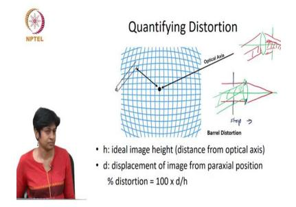
If you will, how do you quantify distortion? Well let us say from this is an optical axis a point should have lain at some position this is the ideal paraxial point the image, but instead of lying here it lies a distance d away. So, the distance from the optical axis the ideal distance from the optical axis if you said that, was h and the extra distance is d then we call distortion just the ratio d by h and it is a percentage. So, it is d by h into 100 ok.
