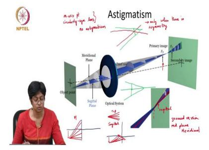
So, we move on to the next monochromatic aberration; which is astigmatism ok. What is astigmatism? And you can see several of you wearing glasses, so I am sure you would have heard the term astigmatism before right ok. So, you have got the idea that; well, this is what every aberration is doing right, different annular zones are doing something, different apertures are doing something.
