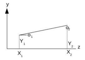
So, let me redraw this diagram. So, this is the optical axis, this is y and let us say I am interested at two different points on the optical axis. So, I have a ray that is coming in here it has height  $y_1$  it is angle is  $\theta_1$  and at some other distance z this ray is now traveling and it has now assumed that is a straight line. So, over here it has continued and at this interface maybe something happens. So, this is  $\theta_2$  and this is  $y_2$  and this is at  $\theta_2$ .
