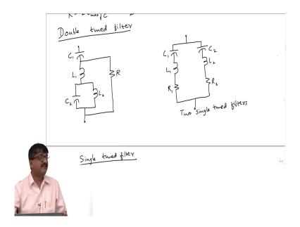
So, I can have instead of two single tuned filters, one double tuned filter.
