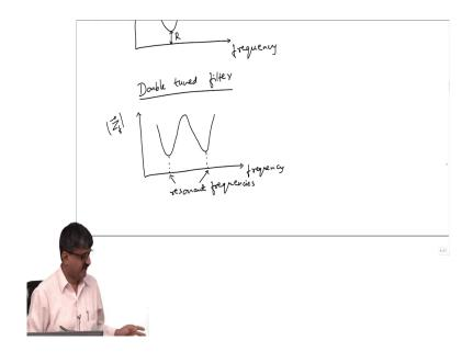
So, again these two values of frequency at which I have minima or known as the resonant frequencies. So, these two are called resonate frequencies. So, what I would ask you to do is, try to get an expression for the resonant frequencies. Of course, one can make an a simplification neglect R; see neglecting R means, what do you meant by neglecting R? R is.
