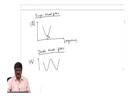
Now, the question is, how is this double tuned filter supposed to behave? See in the case of single tuned filter; see if I take a single tuned filter, suppose I plot the magnitude of the impedance of the filter as a function of frequency ok. So, it is somewhat like this there is at one value, I get a minimum value of impedance. What is that minimum value for single tuned filter?
