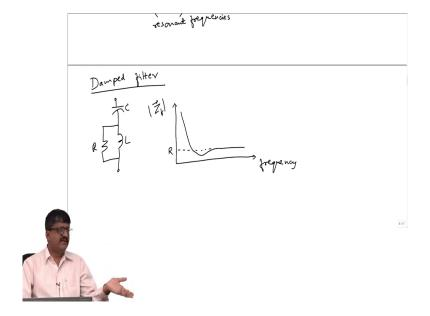
So, it is a high pass filter; that means, all the high frequencies will pass through that. A Damped filter is it like this, it has a capacitance, inductance and a resistance connected across; the inductor, resistance is connected across the inductor. So, if you look at this plot of magnitude of impedance as a function of frequency so, here suppose let me call this capacitance L inductance, capacitance C inductance L resistance R.
