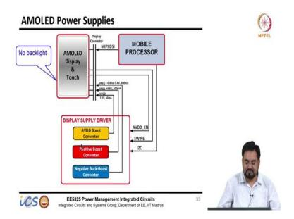
So, AMOLED displays do not require a backlight as we need in LCD and the reason is that it's LED and has its own light. The supply requirement is different for these and what we require again are 3 supplies here just like in LCD, but the voltage levels are different here. We require a negative buck boost or negative supply just like we need in LCD. We require a positive boost also and AVDD is different.
