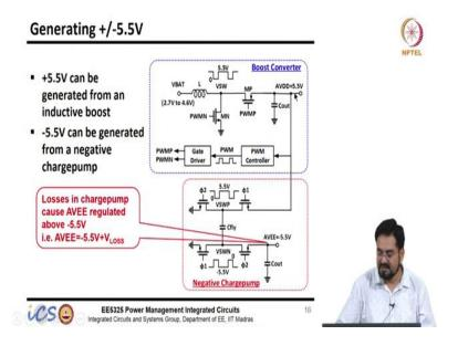
For -5.5 volt, now we have 5.5 volts and we can invert that simply by using an inverting charge pump.
