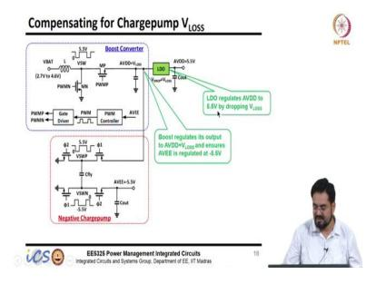
So, in order to get this minus 5.5 volt back, I can regulate this voltage at 5.6 volts so that I can get minus 5.5 volts, and then an extra 100 millivolts I can drop in the LDO. So, your efficiency will be degraded a little bit, but if you have a requirement of exactly the same voltage on both sides then I mean you have to live with that.
