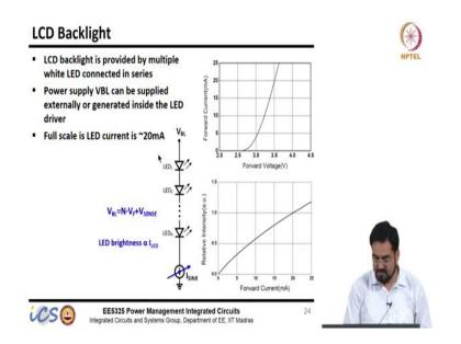
So, backlight requires LEDs and these LEDs have a certain forward voltage, it is not like a normal PN junction diode which has a 0.7 volt, but these are much higher. So, mostly order of more than 3 volts or so. So, if it is a white LED it may be 3.3 to 3.5 volt and with the forward voltage your forward current also changes and these LEDs require constant current because we know that this current has an exponential behavior with respect to forward voltage.
