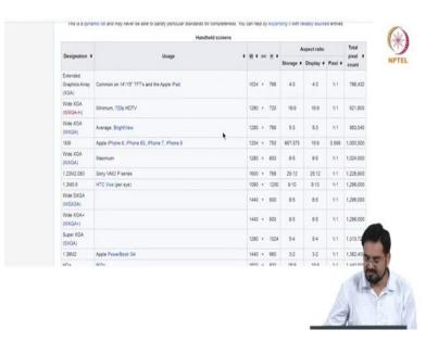
Width over length will give you the aspect ratio and it depends on the shape of the display also. I mean square or rectangular or width is more than height or height is more than width. So, that gives you an aspect ratio. So, you can get a different pixel size in the x and y direction.
