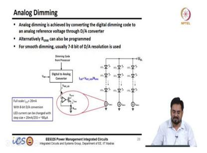
Analog dimming is quite simple, we know we have this sink regulator. All we need to do is change the reference voltage. My current is nothing but this  $V_{REF-LED}$  divided by  $R_{SINK}$ . You have a fixed  $V_{REF}$  and you can have a digital to analog converter to generate a programmable voltage. So, it has to be digitally programmed because the command I am getting is binary
