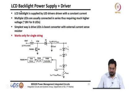
So, the backlight is basically supplied by this boost converter. So, we know that we need to boost this voltage. Let us say that each LED has roughly more than 3 volts. So, 8 LEDs may require roughly 28 to 30 volt,s and in order to get this 28 to 30 volts from battery voltage which is 2.7 to 4.6 volts we need to boost it. It looks like you are boosting more than 5 times here even for the higher maximum voltage. So, when you go to 2.7 volts then that will be even higher.
