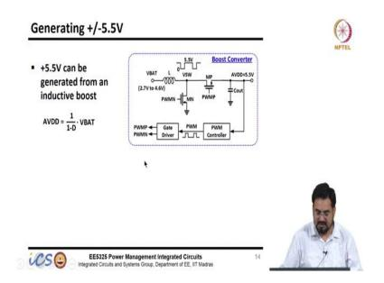
For plus 5 volts, you can simply use a boost converter. So, it is a simple inductive boost regulator and we know the output voltage will be 1 over 1 minus D times into VBAT, where VBAT is the battery voltage which is changing from 2.7 to 4.6 volts. So, based on the voltage control loop will just change the duty cycle and it will keep output regulated at 5.5 volts with variable input supply.
