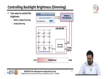
So, now we have these current sinks and they can be programmed. So, that is how you dim your brightness or control your brightness. So, that is what the controlling brightness is called dimming. Changing brightness through the phone does nothing but controls this current and that is how your brightness of the screen is controlled. This current can be controlled in different ways. One way is PWM or digital dimming and the other is analog dimming.
