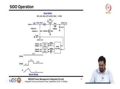
So, you allot half the time to boost and rest next half time to inductive buck boost. So, it is more like multiplexing in time. So, in buck mode, it supplies and one thing is you have to
