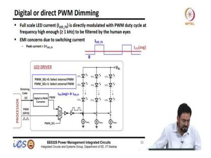
The next one is digital or direct dimming. In the digital dimming instead of programming the voltage, we simply turn on and off the current strings. Let us say this full scale current is 20 milliamps again and depending upon what frequency and duty cycle we are turning on and off. So, it will look continuous to our eyes because our eyes cannot perceive anything beyond 1KHz. It has to be done beyond 1 kiloHertz even though our eyes cannot see anything
