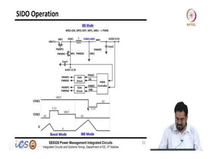
So, there is no issue of cross regulation and all those when your inductor current goes to 0 because it will fully discharge before you activate the next phase or next mode. So, that is how it works, and depending upon the duty cycle the current will change and it will keep the output regulated at plus 5.5 and minus 5.5 volts.
