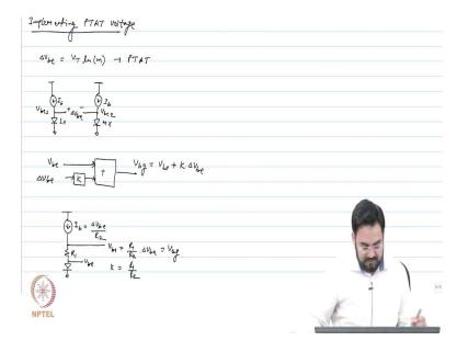
But slopes are different, so you need to scale that. So,  $V_{be}$  is fixed and  $V_{be}$  can't be scaled but  $\Delta V_{be}$  needs to be scaled to match the slope of your  $V_{be}$ . Let's say  $\Delta V_{be}$  needs to be scaled by K. So, we get
