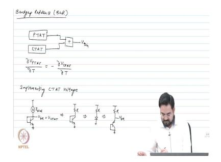
And most of the time we use PNP because in the standard CMOS process we get the parasitic bipolar and you do not get active bipolars.
