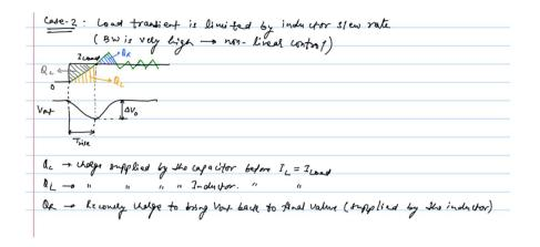
$Q_R$  is the recovery charge to bring the  $V_{out}$  back to final value and it is supplied by the inductor.
