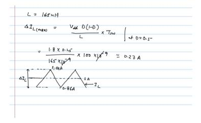
So, we will hit the DCM if load current is  $\frac{\Delta I_L}{2}$ , which is roughly 140 mA.
