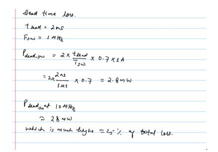
So, at 1 MHz switching frequency dead time switching loss ( $P_{dead-sw}$ ) is 2.8 mW. If you keep the same dead time at 10 MHz, that will be 28 mW which is very high. So, this will limit your switching frequency, or you reduce the dead time proportionally.
