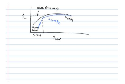
Once you have a PFM mode you will maintain very high efficiency even at light load because you will start reducing the switching frequency. But if you do not have PFM mode then you will get very bad efficiency at light load. For 180nm process and for 1 A current; it looks like 10 MHz is not a big problem, you can easily operate and achieve high efficiency.
