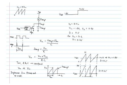
The advantage with feed forward line compensation is it improves your line transient. If there are any fast changes in  $V_{in}$ , those changes will get reflected in your duty cycle immediately and it will not change your output. So, line transient is very good.
