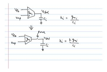
If I modify this  $g_mC$  integrator, let's say I have put a switch, and this is controlled by your PWM as shown in above figure. Then integral gain will be  $K_i = D \frac{g_{m_i}}{c_i}$ .
