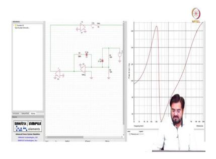
The above image shows the phase response of the loop gain of the converter in the above example with type-III compensation. Phase margin is 75°. At infinite frequency, the phase will go to 180° because we also have an ESR zero which is at a very high frequency.
