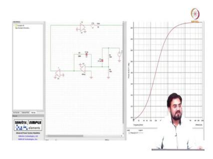
The above image shows the phase response at  $V_{\mbox{\tiny ctrl}}$  i.e. the phase response of Type-III compensator.
