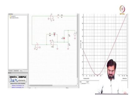
The above image shows the magnitude response at  $V_{ctrl}$  i.e. the magnitude response of Type-III compensator.
