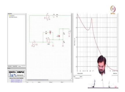
The above image shows the magnitude response of the loop gain of the converter in the above example with type-III compensation. UGB is around 110kHz.
