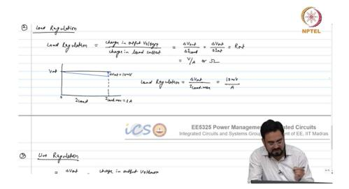
We do not want output to change when the load is changing. Ideally, I want  $R_{out}$  to be zero and that's why we say like ideal supply has zero output impedance, that is what it means because it will give constant voltage across any load current. Ideal and non-ideal plots are shown in the above figure with an example. And blue curve is non-ideal.
