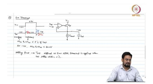
We will take an example of this linear regulator. When  $V_{in}$  changes, this past transistor will create a  $V_{gs}$  difference because this gate voltage cannot change instantaneously. So, the current in the output will increase and this will try to overshoot.
