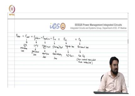
The total loss in DC-DC converter is the summation of conduction loss, gate drive loss, dead time loss, hard switching loss, magnetic loss, and Quiescent loss.
