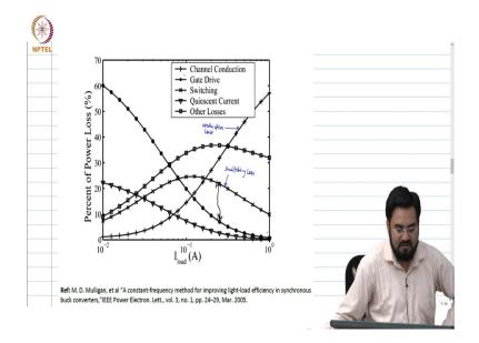
The graph in the above image shows the normalized loss which means it tells the percentage of each loss at different load currents.
