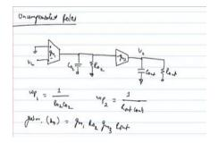
• Pole locations of a 2-stage Miller-compensated amplifier, as shown in the figure:
