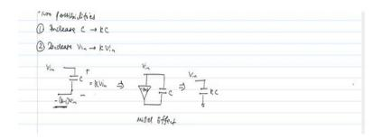
• A common-source amplifier (which is inverting and has a gain of  $-g_m R_{out}$ ) with a capacitor in feedback can be used for Miller compensation.
