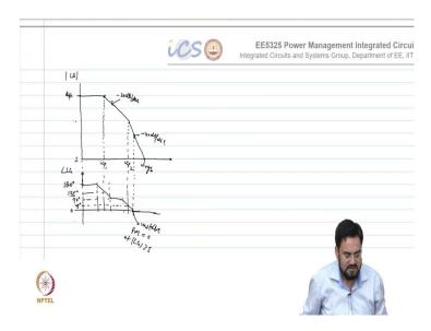
So, you are hitting gain 1 at higher frequency but your phase has already crossed 0°. Which means your system is unstable because phase margin is 0° at loop gain greater than 1. As long as this 0° phase happens before your  $\omega_{ugb}$  your system is unstable. If this 0° phase would have happened after  $\omega_{ugb}$ , then you could have achieved some phase margin and that is what we try to do. Which means your second order system has a tendency to become unstable.
