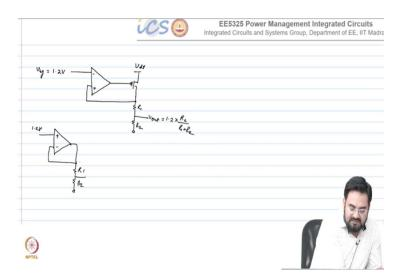
If we directly use the resistor divider, then the problem is this resistor divider will load your previous stage and this may disturb the band gap voltage. So, you have to use a buffer as shown in circuit diagrams.
