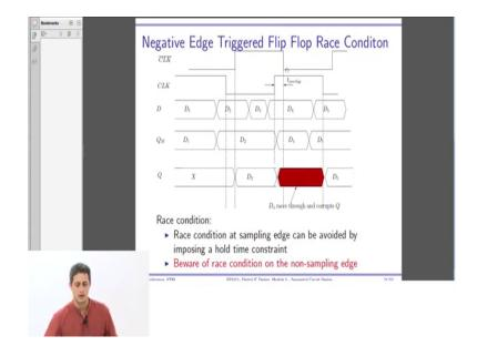
This was the non sampling edge this is a negative thing right; this non sampling edge because of the overlap had to have some constraints there. And what was the constraint it basically said that the overlap period should be smaller than the delay of going through this, pass transistor through this, inverter through this, pass transistor. And know you are getting there that was an implicit condition in the flop design.
