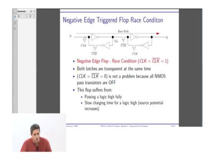
So, its not with the condition vanish, the condition is implicitly there. There are still three conditions but one is one is something a designer does not have control over it has to be taken care of at design time or the flop itself. If I give you the flop that internal race condition constraint is already fixed you can do nothing about it. Whereas, in a latch base system, I can do something about it because C 1 and C 2 are still in my control clear.
