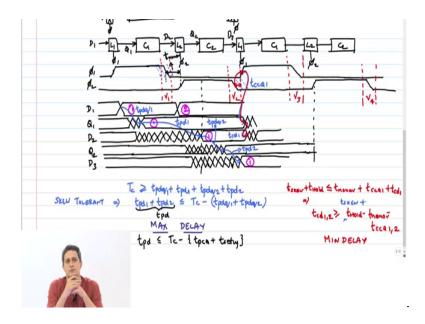
So, let us just revisit the latches max delay and min delay constraints ok. So, what is my constraint let me just go to the new page; because I need more space I have latch L 1, combinational block C 1, L 2, combinational block C 2. Now instead of going to L 3 I am going to bring back L 1 ok. Physically in space this is not a L 1 I am actually unrolling this in time.
