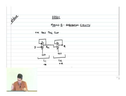
So, let us move on with our discussion and in the last class we discussed the construction of a master slave flip flop, right. Using two latches in order to get a positive edge triggered flop we said you need it to, right. So, clock we needed a negative latch first which means that this has to be 0, this has to be 1, D can go out to QM, right.
