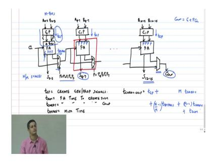
So, each block I first need to create the generate and propagate signals right, that is going to take one unit of time. So, that is the first block that I will put G P and this is going to take 4 bits A 0 to 3 and B 0 to 3. Then I have a full adder and then what I am going to do is it this is my C in, I want to put a BYPASS MUX here CARRY out will come from here and C in will come from here, this is my propagate signal P equals P 0 P 1 P 2 and P 3 ok.
