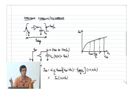
So, if I have an a logic inverter driving a load capacitance right this inverter is going to either charge this capacitor or discharge this capacitor, and the delay of the gate is determined by how fast this action can happen ok. So, I also told you that delay is defined as the time it takes for the input to go to 50 percent right from there till the time the output reaches 50 percent ok.
