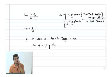
So, let us look at this equation a little more closely R equivalent is 3 by 4, I leave out this lambda parameter I naught ok. If it is velocity saturated then I naught is equal to K n prime W by L V D SAT n into V DD minus V Tn minus V D SAT n by 2 ok. If it is a long channel device and it enters saturation region then it is just K n prime W by L into V G V DD minus V T whole squared and half right.
