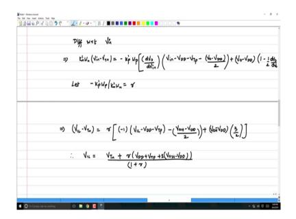
Then I can say implies V in minus V T n equals r times dV out by dV in. What is dV out by dV in? At that point minus 1 right; so, therefore I can write this as minus 1 and what is V in at that point V IL at that point when the slope is minus 1, there by definition it is V IL right into V IL minus V DD minus V TP minus V OH minus V DD by 2 right.
