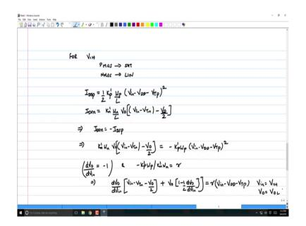
Now what about V OH V OH? You got to do the exact opposite right. For V IH PMOS is in which region? Saturation NMOS is in linear, ok. So, can we write the expressions of the currents ids p is K p prime half W p by l into V G s minus V T p the whole square right which is nothing, but V in minus V DD minus V TP whole squared and ID S n equals K n prime W n by l. What is V DS for the NMOS? Yeah V naught. What about V in minus V T n minus V naught by 2, right.
