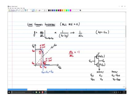
So, let us go back to long channel inverters which means that all short channel effects equal to 0. No channel length modulation, the velocity saturation voltage is very high right. So, therefore from linear it will only go into saturation right and all these things basically just vanish from our discussion ok. So, now if you remember the gain expression right equal to dV out by dV in at V in equal to V out equal to V m was proportional to 1 over lambda n minus lambda p, right.
