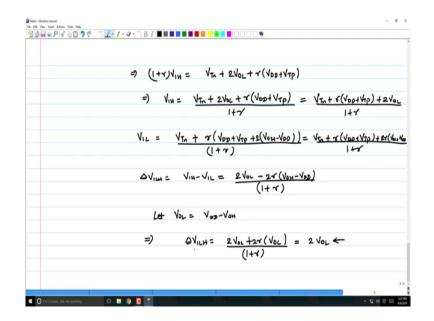
So, for example you could assume let right V OL equals V OH minus V DD or V DD minus V OH for symmetry, right. It is on either side. It is going by the same amount is what we are saying. So, if that is the case, then what does that thing simplify to V IH is 2 V OL minus plus 2 r into V OL, sorry right. What is it simplify to 1 plus r comes out and you have twice V OL.
