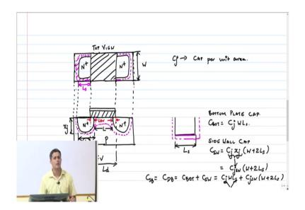
So, what is my perimeter capacitance or rather it is called side wall capacitance for obvious reasons ok; this is called bottom; bottom plate CAP or bottom wall does not matter ok. So, side wall CAP is again going to be C j ok; side wall C sidewall is huh? Exactly, it is going to be x j into what? W plus 2 L S right because this dimension is L S and this other dimension is W; total perimeter we are talking about is W plus 2 L S.
