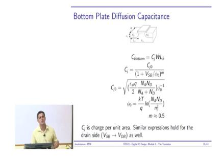
So, it turns out that the capacitance per unit area is as shown here. Let me just; maybe I can just write it down capacitance per unit area; k is equal to C j naught is what? Root of epsilon
