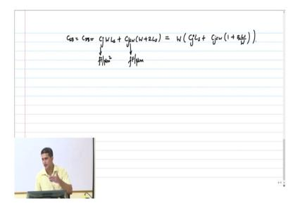
So, the total capacitance C SB equal to C DB is equal to C j into W L S plus C j S W into W plus 2 L S. Yeah, no my question I ask you is like I combined this into C j S W; why cannot I combine C j into L S and give you one number; say that that also I will make it as capacitance. Because now look at what is happening this guy is femto Farad per micrometer square capacitance per unit area.
