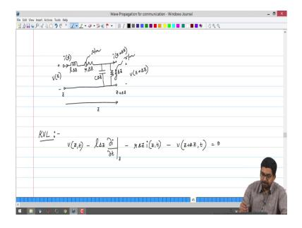
So, I have a series inductor just as we had seen in the prior classes ok and we had a resistor in the series path ok. In the prior lectures in the lossless transformation line, we had connected a parallel capacitor in the model. Assuming that there is a conductive path across the capacitor, a conductor is added in the parallel path also.
