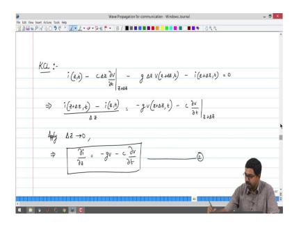
The same way we can apply KCL for the incoming and outgoing currents in the section. If the incoming current is considered as positive and the currents that are leaving this transmission line section are considered to be negative, we can start with
