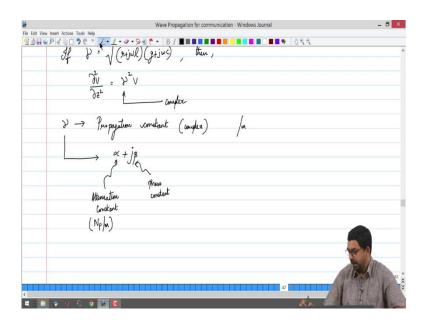
It is composed of a real and an imaginary part and to denote that we write it in the form of a complex number  $\alpha$  + j  $\beta$ .
