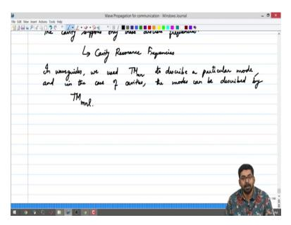
Just like in the waveguides we used in waveguides we used TM say mn to describe a particular mode, whose cut off frequency can be calculated by using the field descriptions that we had before.
