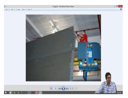
So, you can have a look over here all right. This is how an array of antennas will be connected to array of detectors using some waveguides. So, you have large number of 90 degree bents going on all right. It means some kind of an array detector and the energy is going to some place where it is going to get converted into say electric signal and then you are going to make an analysis.
