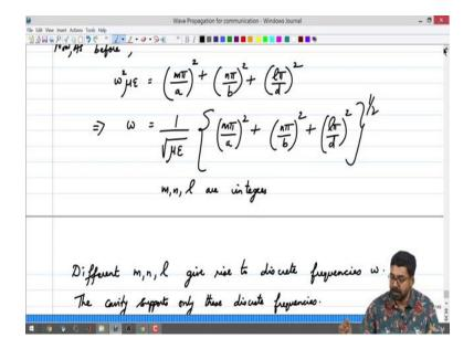
And just like before we can also make a few statements m n l are integers m n l are integers. So, different values of m n and l can be substituted in this expression for a given cavity geometry which has the sides of a centimeters by b centimeters by c by d centimeters extra.
