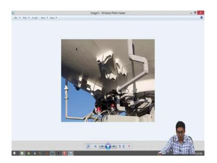
So, this is in practice. So, on top you are seeing the antenna all right there is a giant dish antenna over here and from the antenna all right, there is a waveguide that is coming into the picture it is being bent being bent again and it is being sent to some units which are going to detect and do some processing this is from a radar ok.
