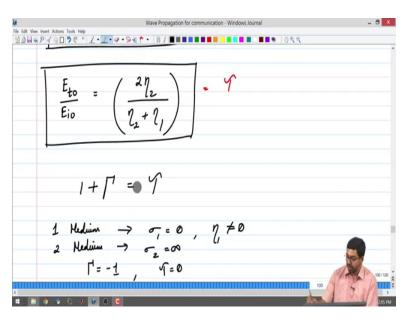
And there was a relationship between the transmission and reflection coefficients ok. And we found that  $1 + \Gamma = T$  all right. This means that the transmission coefficient can be greater than 1 when we are talking about the value of the electric field all right. So, it means that your incident electric field can be 1 V/m, the transmitted electric field can always be higher than that, but it does not mean that the energy conservation is violated.
