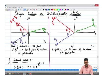
We will get started right. So, I think we are going to start with ok. We are going to look at Oblique Incidence on dielectric dielectric interfaces for this class ok and I am going to divide the page into two columns for two different configurations ok.
