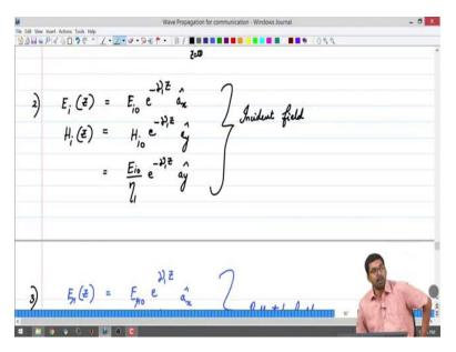
And the transmitted wave, the assumption was that there is no change in any polarization and then we calculated what is the value of a reflection and transmission coefficients. And we found that it looked exactly the same as what we got in transmission lines except that in transmission lines we did not calculate transmission coefficient, we calculated only the reflection coefficient right.
