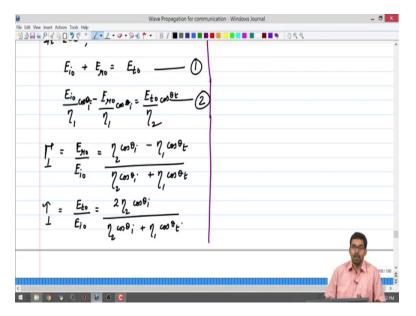
So, in other words you can solve these 2 equations simultaneous equations and you can write down  $\Gamma$  which is nothing, but  $E_{r0}$  divided by  $E_{i0}$  ok. The solution looks like
