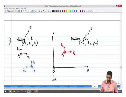
So, we have an axis which is the x axis here, z axis here and to form a right handed triad we had a y axis marked in this way. We talked about a specific case where the polarization of the incident wave was having an electric field component in the plane of the diagram, and the magnetic field was perpendicular to the plane of the diagram.
