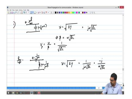
One of the things that we heard earlier learned or begun with in transmission lines is the circuit model of a section of a transmission line. And, we drew a series inductor for a lossless section ok and we had a parallel capacitor alright. And, then we had j $\omega$ l to be the series impedance right and your parallel admittances is again j $\omega$ c, this is what we had before alright. From here we could always find out
