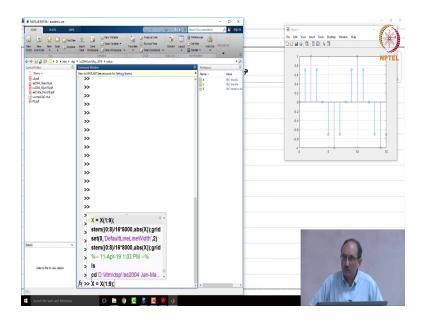
And then, we looked at the spectrum and the DFT in matlab is implemented using the FFT algorithm, we are going to talk about the fft algorithm after this. And because of the symmetry, it is enough if you retain only the samples from 0 to N/2. So, we retain samples from 1 to 9 and remember, matlab is 1 based whereas in all our equations, we mean using 0 based index. Therefore, if you want to use matlab's index, you have to convert that from 1 base to 0 based.
