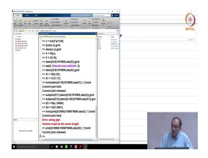
So, this exactly what I did. X2 is what I have plotted, X2 is fft(x, 10000). So, the total length is 10000; the first 16 samples are the samples of the sequence that I generated, the remaining are zeros. And then, I computed the 10000 point DFT and then I took the first 5001 points, which corresponds to the index in the range 0 to 5000 and then I have plotted it and I have plotted using plot rather than stem.
