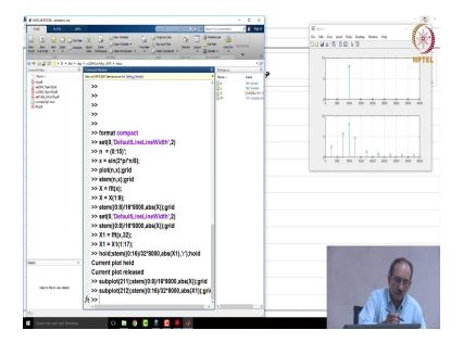
All right, let us get started. We were looking at a matlab example in last class and the signal in question was this. So, this is nothing but 1 kilo Hertz sine wave sampled at 8 and we are looking at 2 cycles here. So, this is the plot of the time domain sequence, you can also show this as a stem plot which is more typical.
