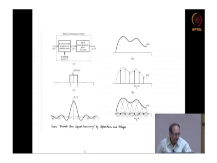
So, we see if I can, if this is. So, this is the underlying continuous time signal. These are the samples. Each sample elicits a sinc response like this. The only difference is the location of the sinc and the amplitude of the sinc. Note that, when you consider this particular sinc, every other sinc goes through zero crossing at that point. In between, they all add up to give you the exact curve without any loss of information. So, this is how the theoretical construct behaves.
