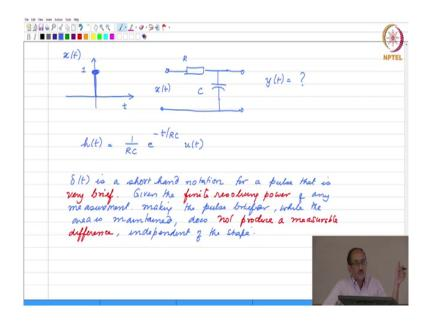
So, this is x(t) and then this signal is applied to this circuit. So, R can be anything, it can be  $1\Omega$ , C can be 1F. So, this is my x(t) and then the question is what is y(t)? The impulse response is
